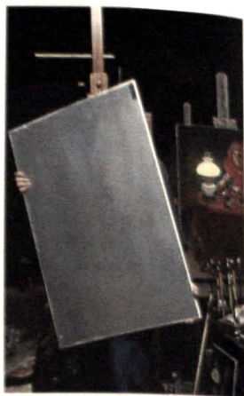
A honeycomb aluminum panel as seen from the back. Canvas is glued to the front of this panel with a removable conservation adhesive. The rigidity of the panel should effectively mitigate the forces that cause cracking in oil paintings.
